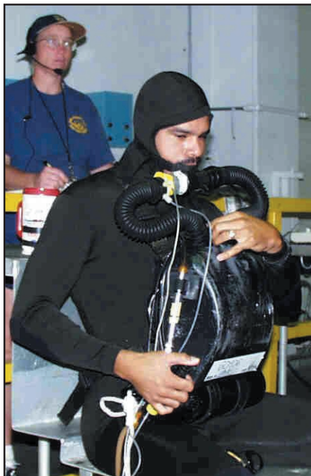
Preparing for an instrumented experimental dive in 99° F water.
