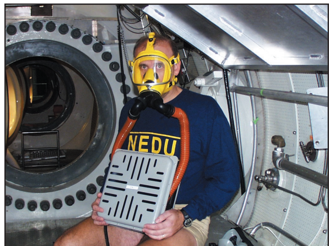
Breathing a MK 18 Escape Breathing Apparatus (EBA) during a 2-hour saturation dive to develop emergency decompression schedules.
